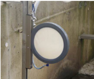
The P700 filter mounted inside a tank. Easy to clean with water and a brush, bleach, or hydrochloric acid.
